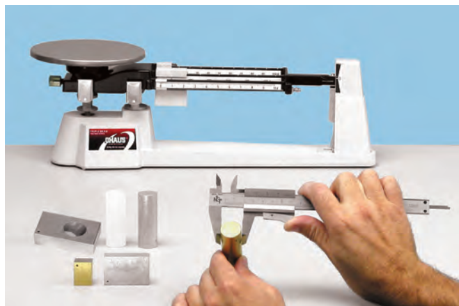
The mass and volume are measured to determine the dependence of the buoyant force on mass, volume, and density.
