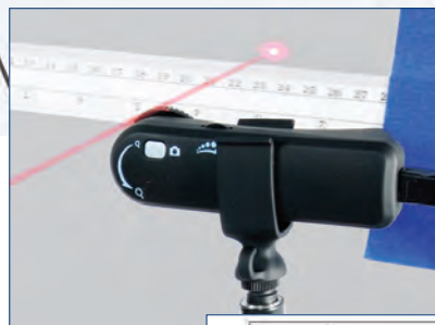
The USB Camera Microscope (not included) records the oscillation of the laser beam.
