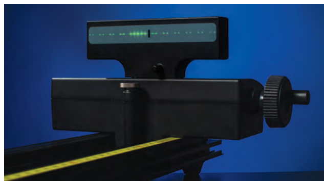
The laser interference pattern is scanned by turning the crank.
