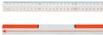
The Four-Scale Meter Stick is an important part of the Significant Figures Kit as it includes four scales of varying precision.
