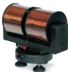
Electromagnet produces about one Tesla.
