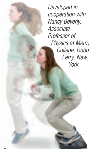
The normal and parallel forces are recorded as the girl jumps off the platform.
