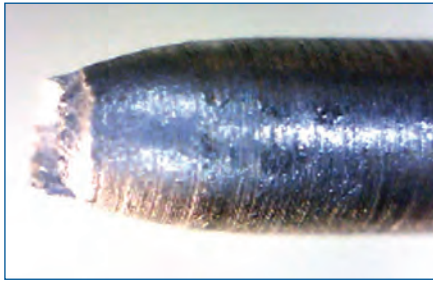
Image of broken steel tensile sample taken with a microscope.
