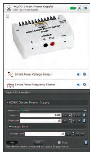
The AC/DC Smart Power Supply is controlled in PASCO Capstone or SPARKvue software.
