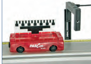
Position and velocity graphs are obtained using a Picket Fence and Photogate.
