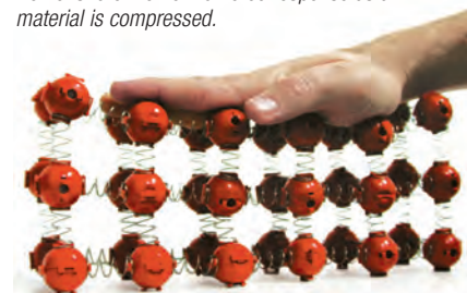
Demonstrate the normal force response as a material is compressed.
